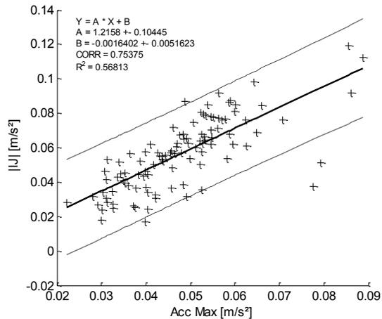
Fig. 6: Correlation between amplitude of the IJ wave and the maximum of the magnitude of the acceleration vector for the BCG recording of the Spacelab-D2 experiment.
