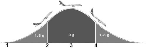
Fig. 2. Typical flight maneuver during a parabola obtained with the Airbus A300-ZéroG of NOVSPACE [15]. A parabola is divided into the following parts: 1) "Pull-Up", 2) "Injection", 3)  $\mu$ G and 4) "Pull-Out".
