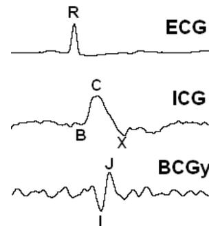
Fig. 1. Illustration of the characteristic peaks defined in the ECG, ICG and BCGy signals. The R-peak in the ECG was used as reference point to measure the time intervals. The C-peak is the maximum of the first derivative over time of the ICG. B and X points represent the opening and closure of the aortic valve, respectively. I and J peaks are two extrema of the BCG.
